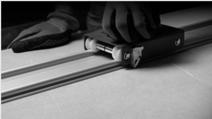
CUTTING DETAIL WITH GUIDE ON SLAB
